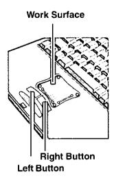
Use the touch pad to move the cursor on the display and perform normal computer operations. For instructions on how to operate, refer to Reference "Touch Pad (Advanced)".
